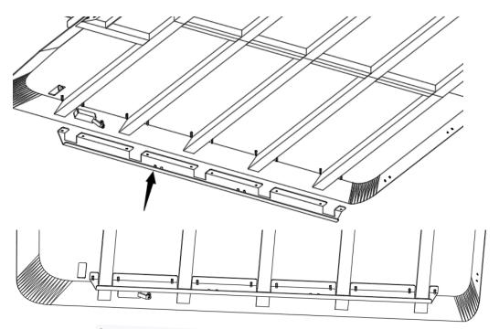
Align the holes of the longitudinal braces with the longitudinal rod
