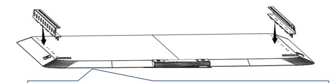
Insert the screws under the upper vertical rod into the holes in the upper cover
