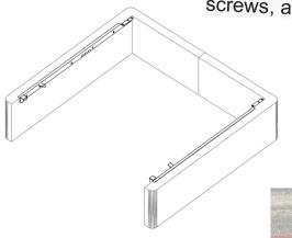
Install the lower bracket. If there are no suitable holes, you need to drill holes. Use cylindrical head  $${\rm M8x}{30}$$
