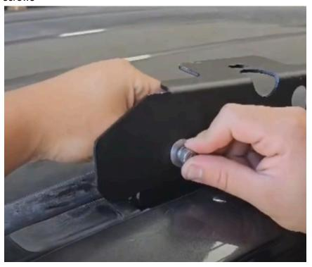
Add the channel nuts with the nut screw to the long backbone
