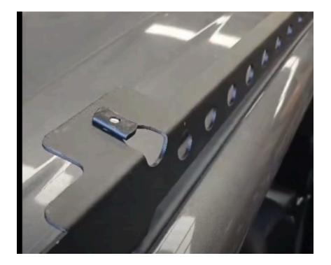
Use the bolt screw with the channel nut to secure the platform to the backbone
