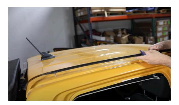
Assemble the roof rack with the backbone and small brackets then ask someone to help you place it on the roof so you know exactly where you want to install it. Once lined up mark out where you will drill ( away from the airbags)
