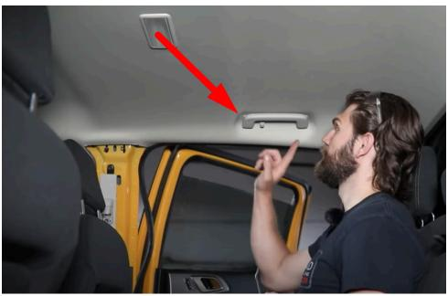
Beware of drilling into the airbags when drilling roof holes
