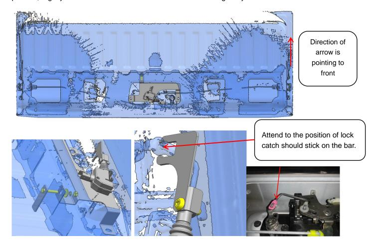
Install the steel cover plate back to the tailgate after the installation, wiring harness connection and testing. The ways of wiring harness connection show below.
