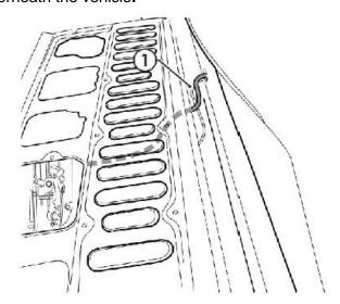
2. Route the wiring harness along the chassis rail to the driver seat.
