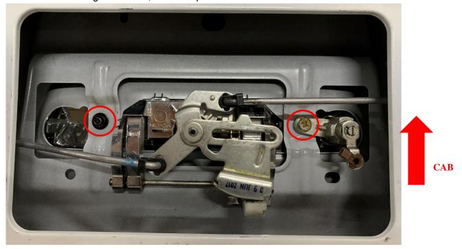
Install the bracket assembly into the tailgate, fasten it with the two original screws mentioned above. Install 3 bracket 3 and fasten it with 8 9 1:
