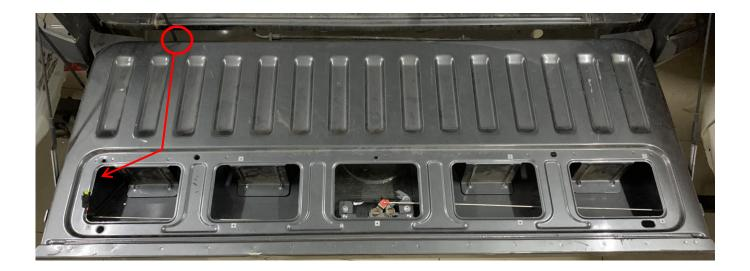
Connect the wiring to the ③ actuator
