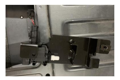
As below picture shows, put the bracket assembly inside of the tailgate.
