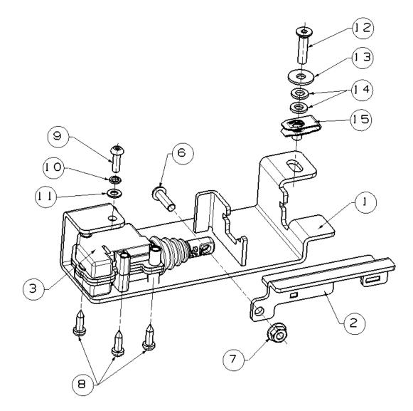
As below photo shows, install ① bracket 1, ③ actuator ① Clip Nut M6 with ⑧.
