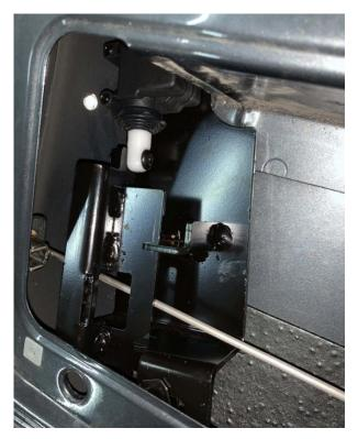
Adjust the bracket assembly to appropriate position, test the locking function. Then reinstall the cover plate on tailgate.
