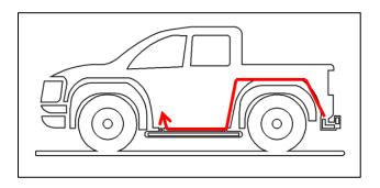
Run the wire harness from tailgate to fender flare through chassis.
