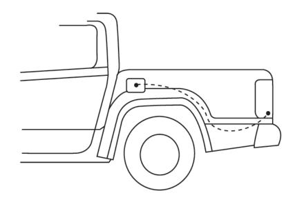
3. Remove indicated fuel cap wiring cover.
