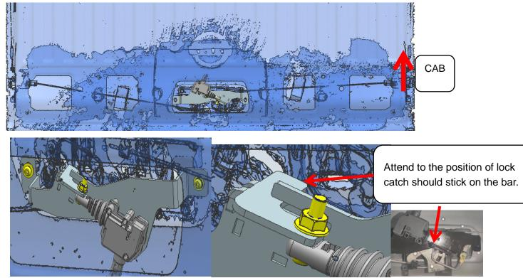
Install the steel cover plate back to the tailgate after the installation, wiring harness connection and testing. The ways of wiring harness connection show below.
