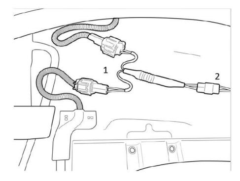
Finish all the installation, test the tailgate lock function with the remote control, after testing reinstall the fender flare and tailgate cover.
