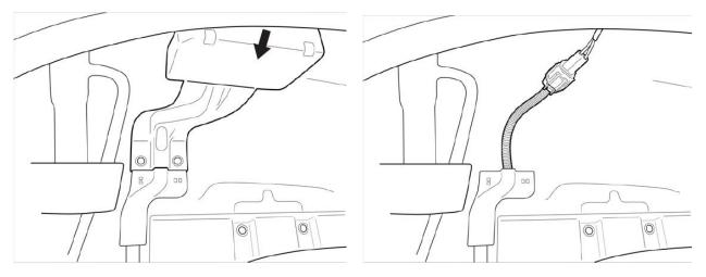
4. As below picture shows, connect the OE wiring with (5) (the wire harness we supplied).
