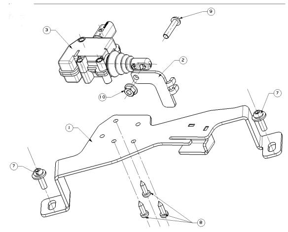
Installing the lock assembly, refer to the diagram above, Combine ① Bracket 、② Locking plate、③ Actuator with ⑧ Phillip tapping screw ST4.8\_16 ⑨ Hexagon Socket Button Head Screws M6\_25 and ① Hex flange nut M6.
