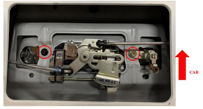
Install the bracket assembly into the tailgate, fasten it with the two original screws mentioned above. Install ③ bracket 3 and fasten it with ⑧ ⑨ ①:
