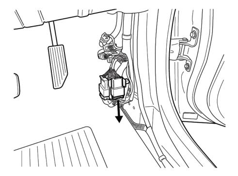
4. Connect the (5) wire harness 2 to vehicle harness. Also connect the other plug with the (4) wire harness 1, then press the key fob to check the tailgate locking function.
