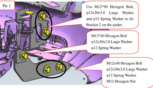
Step 3: Install the front guard on the brackets and then adjust them to the proper positions.
