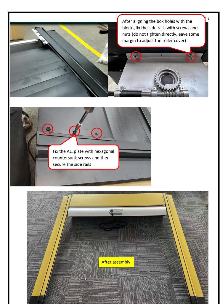
3.Place the assembled manual roller cover tightly against the inner side of the car on the carriage, measure the front and rear spacing of the two side rails with a ruler, and ensure that the side rails are placed in the middle of the carriage, with consistent spacing required
