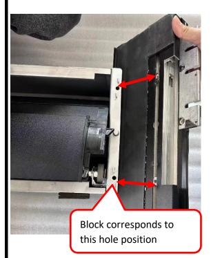
Pull out some of the roller and then snap the side rails into the roller
