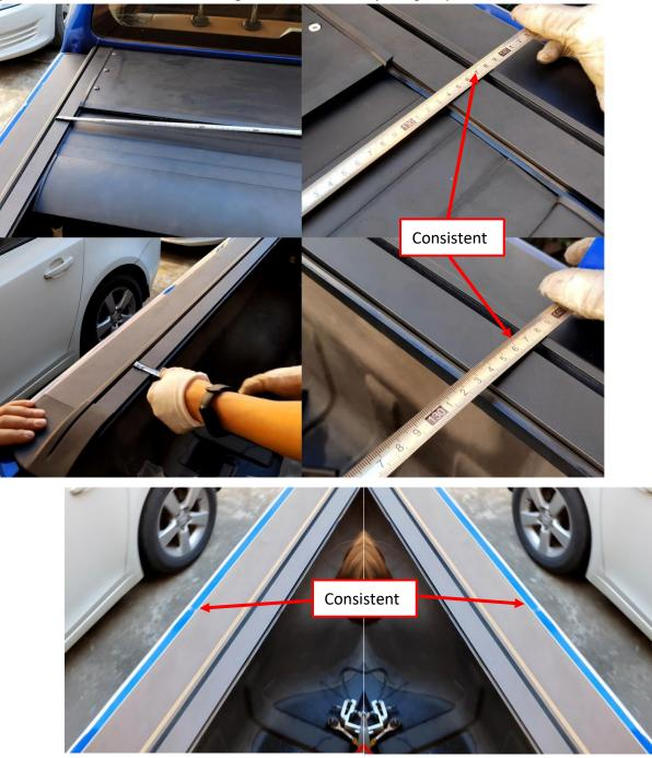
4.Slide the block to the appropriate position and install the screw
