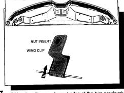
7. Slide wing clips over bonnet edge at the two previously noted outer positions.
