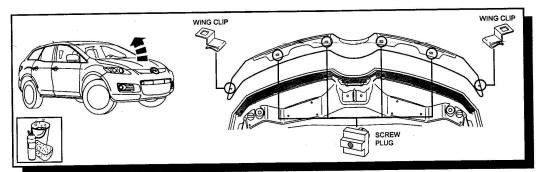
Open & clean the bonnet. Trial fit the Bonnet Protector centrally onto bonnet. Note the rubber seal on the underside of the bonnet. Note the slots in the underside of the Bonnet Protector tags that correspond to the plugs in the rubber seal. Also note the wing clip slot positions with bonnet lip, and mark the centre location of these slots on the bonnet with a pencil or non-permanent marker. Remove Bonnet Protector.
