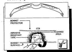
Clean the noted areas under the wing clip locations with alcohol wipe provided. (see step 1) Wipe off any residue with a dry clean cloth. Adhere the abrasive resistant tape strips over the bonnet lip. Apply tape so approximately half of each strip is adhered to the topside and half is adhered to the underside of bonnet.
