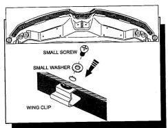
8. Secure Bonnet Protector to wing clips with the small screws and small washers provided.
