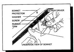
Insert the self-tapping screw and large washers into vacant holes in the rubber seal. Position the rubber seal over the Bonnet Protector tags. Maintain thumb pressure against the underside of the Bonnet Protector and rubber seal, then insert the screw into the screw plug. Ensure the Bonnet Protector is centralised on bonnet then tighten screws. IMPORTANT: Thumb pressure must be maintained to prevent the screw plug from rotating. DO NOT OVERTIGHTEN SCREWS.
