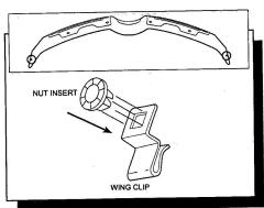
6. Position the nut insert into wing clips.
