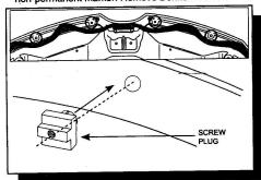
Remove the corresponding plugs from the rubber seal, then install the screw plugs into the vacant holes, as shown. Retain rubber seal plugs for possible future use.
