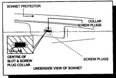
3. Centrally re-fit the Bonnet Protector, locating the Bonnet Protector tags between the rubber seal and the bonnet. Fit the Bonnet Protector tag slot over the collar of the screw plug. Important: Ensure the slot is centrally located over
