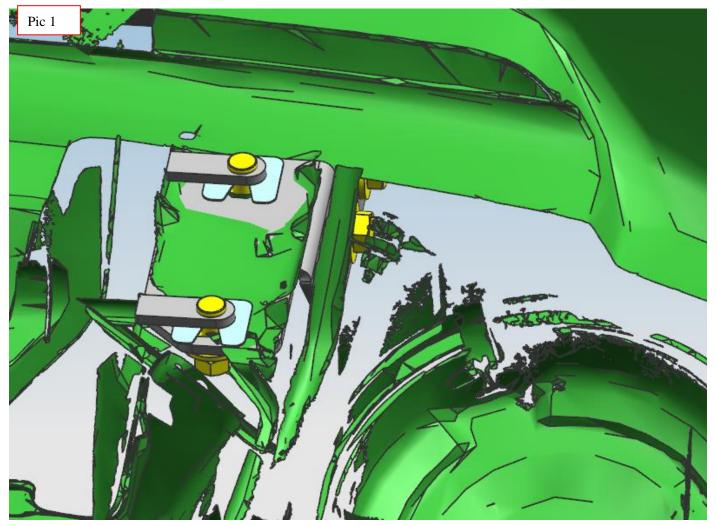
Step 3:Install the bar body on the bracket and adjust the mounting position of the bracket according to the position of the bar body.
