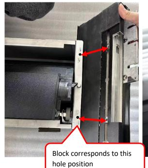
Pull out the roller and then snap the side rails into the roller
