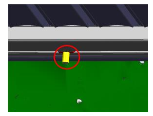
5.Install the bracket at the corresponding position of the screw, fixed with a hexagonal flange self-drilling self-tapping screw on the tub.(The contact surface between the brackets and the side rails should be flush.) and then fixed the bracket and the side rail with hexagonal flange nuts.
