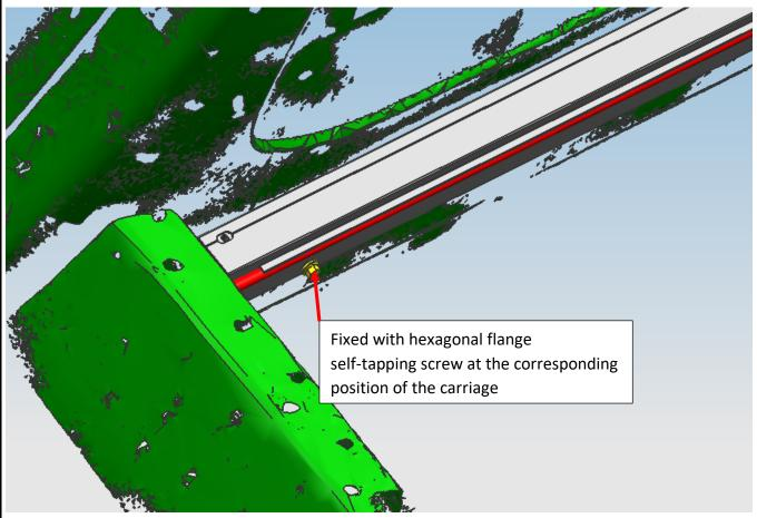
3.Put the assembly roller lid to the carriage, measure the distance between the left and right side rail to ensure that the roller lid is placed in the middle of the carriage.
