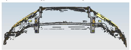
Step 3:Install the nudge bar on the bracket and adjust the mounting position of the bracket according to the position nudge bar.
