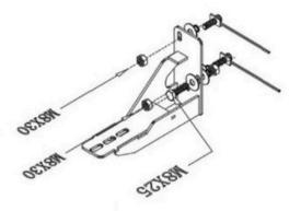
2. Refer to the figure below to install the bracket
