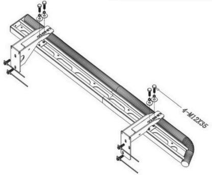
3. Refer to the figure below to install the side guardrail (Note: Only one corner or side guardrail can be installed)
