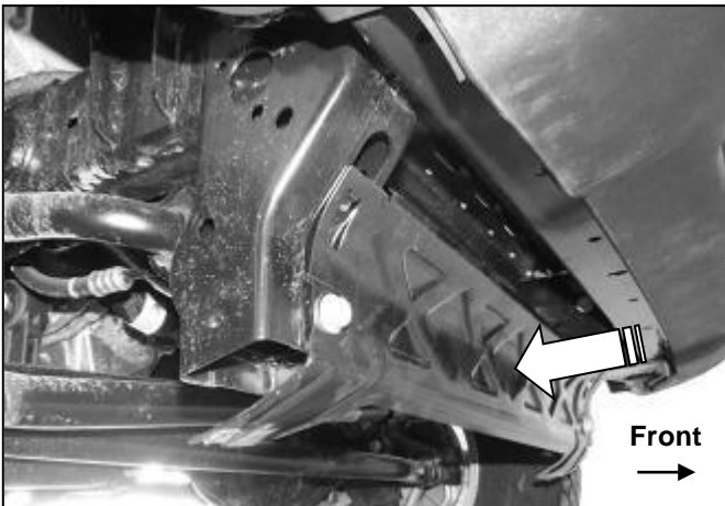
(Fig 1) Remove splash guard and bracket (arrow)
