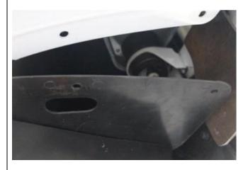
Remove the outside splash guard bolts, (1 x bolt, 2 x plastic buttons per side) and allow guards to hang down.
