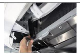
Remove the two bumper support brackets (1 per side, 2 x bolts per bracket). Remove the outside chassis bolts, one bolt per side,
