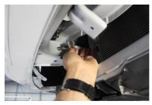
5) Slide flat washer, square washer and tube spacer onto M8 x 100 bolt. Fit bolt assembly (from inside of chassis) through existing hole and through alloy mount plate. Fit 8mm flat washer, spring washer and nut. Align bar with vehicle and tighten bolts.
