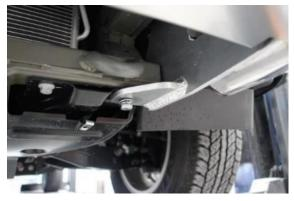
4) Fit bar and loosely secure using M10 bolts through bottom mount brackets.
