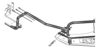
$\tau$  (Check whether the lever body is installed in place, and tighten all the screws to complete the installation.)
