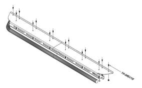
6. . (Refer to the figure below to connect the side guardrail and the front bumper body(Note that after matching the appropriate position, mark and punch holes on the 47 round tube).)
