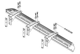
. (Refer to the figure below to install the side bar corners (note that only one corner or side guardrail can be installed).)
