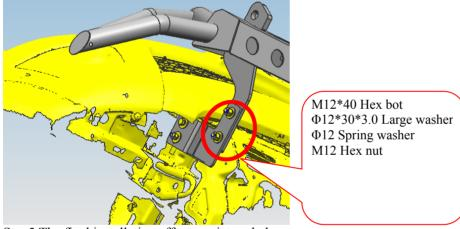
Step5:The final installation effect as picture below:
